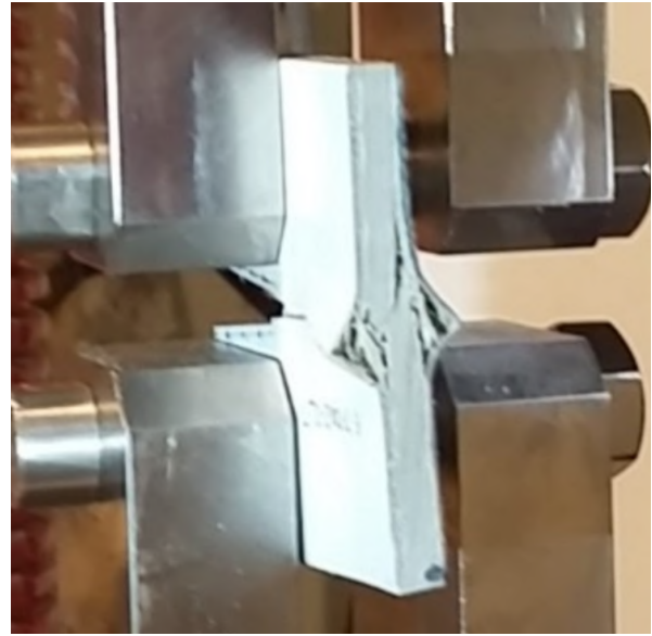
Figure 3.13: Compact tension tests - experimental results: (a) representative load vs. CMOD curves; (b) delamination due to compressive stresses in a I152-CP specimen. Source: [44].
