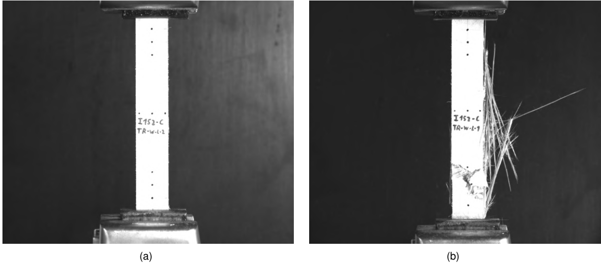
Figure 3.2: Experimental setup of tensile test from I152-CP-W: (a) initial setup; (b) failure mode of a longitudinal specimen. Source: [44].
